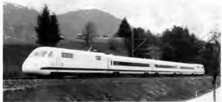
The German ICE will enter service in 1991. Speeds of up to 300km/h are planned and a speed of 406.8 km/h has been achieved. — Deutsche Bundesbahn photo.
