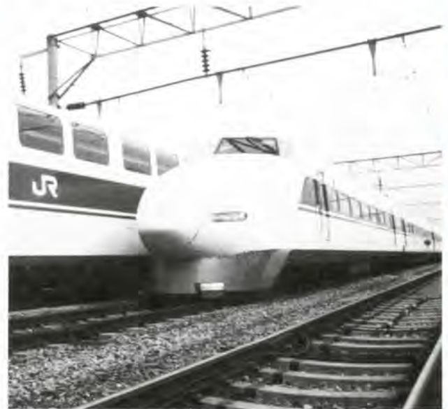
Shinkansen trains introduced modern high-speed rail travel in 1964 with cruising speeds of 210km/h
